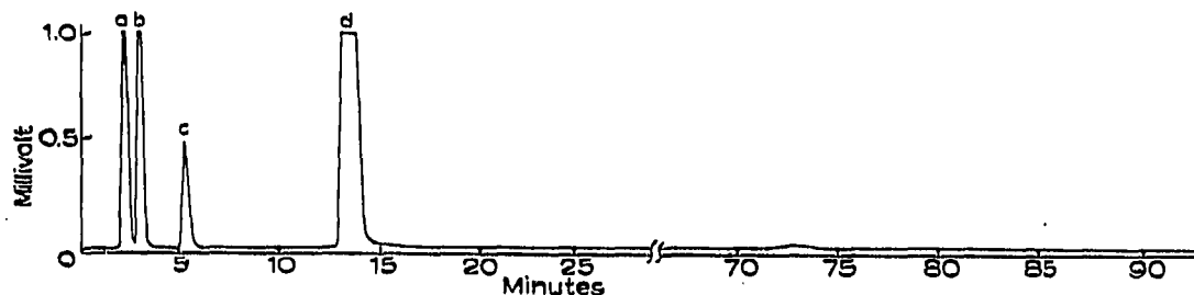
Fig. 10. Microhydrogenation of pyrolysis products from neoprene. Chromatographic and pyrolysis conditions: same as Fig. 6. Hydrogenation conditions: same as Fig. 7. Sample size: 0.13 mg. Identification of hydrogenated products: a = methane; b = ethane; c = propane; d = n -butane.
